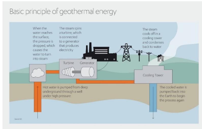
**Figure 1.** The basic principles of geothermal energy
