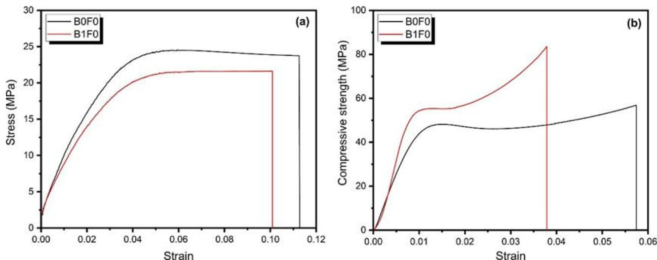
Figure 3. Mechanical properties of the samples: (a) Tensile strength, (b) Compressive strength.
