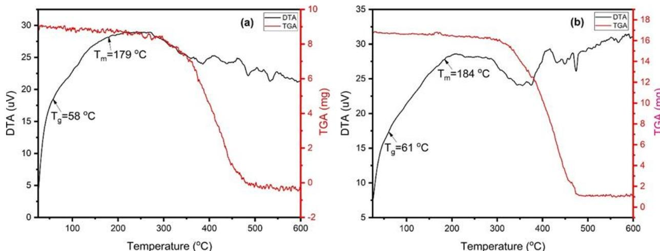
Figure 2. DTA/TG analyses of samples; (a) PLA, (b) 1 wt%  $H_3BO_3$ -doped PLA
