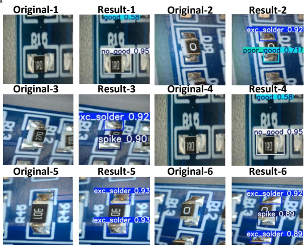
Figure 6. Visual examples of YOLO-v11s model on PCB test data.
