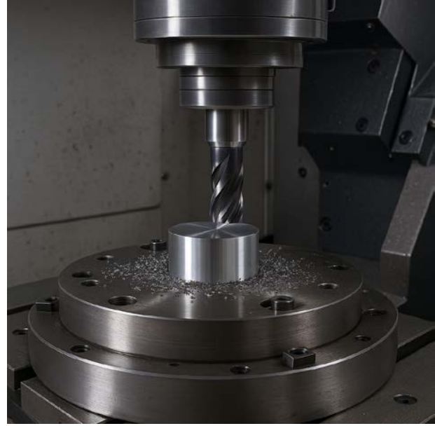
Figure 1: Vertical milling machine performing face milling operation (CNC machining process)
