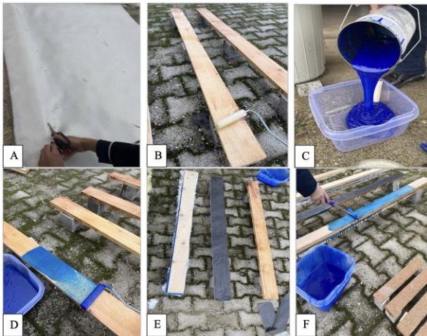
Figure 2. FRP application stages (A) Sizing the FRP fabrics, (B) Applying primer to the surface, (C) Pouring the epoxy adhesive into the mixing container, (D) Applying adhesive to the surface, (E) Placing the FRP fabric on the surface, (F) Applying the same application to the second intermediate layer
