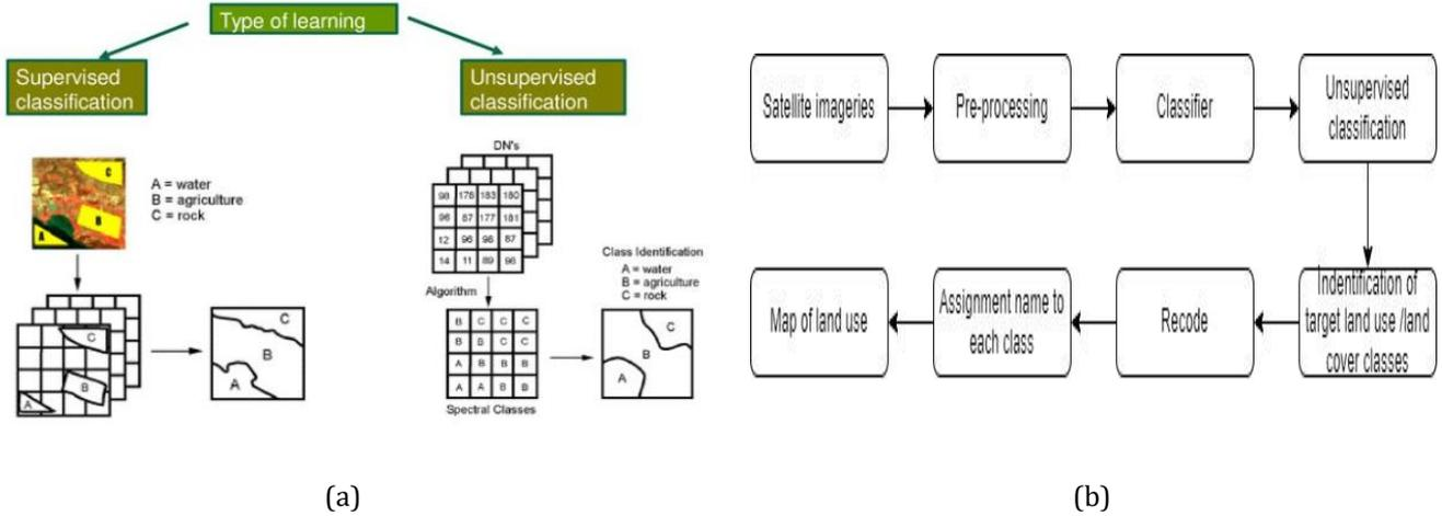
Figure 3. (a) Unsupervised classification (ESA, 2009) (b) Unsupervised classification workflow diagram
