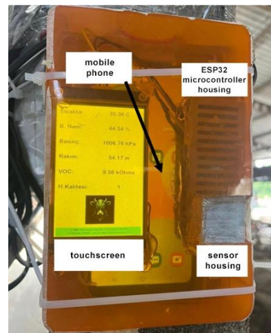
Figure 2. The prototype device and its components
