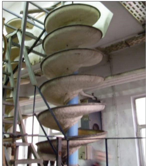
Figure 2- Reichert spiral unit in the experimental studies.
