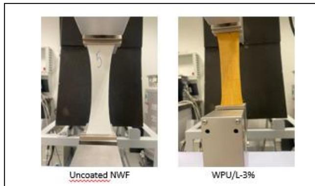
Figure 3. Photographic images of NWFs during tensile test.
