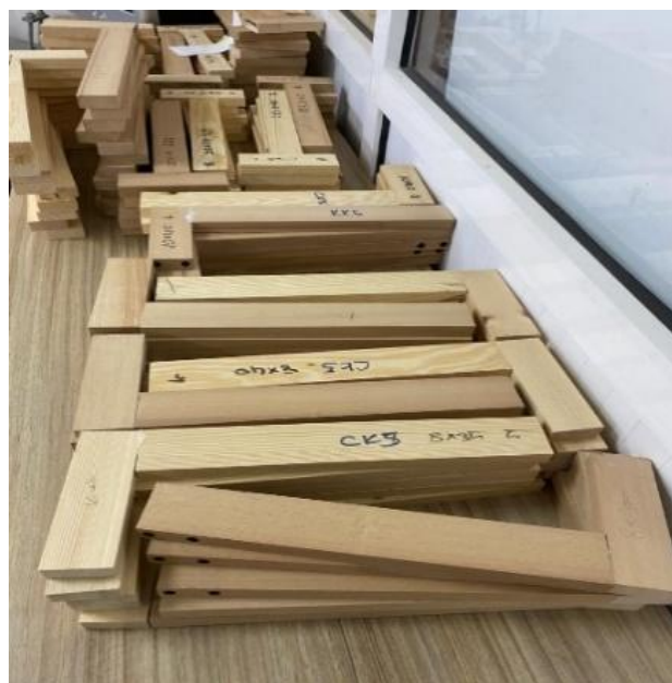
Figure 2. View of the prepared T-type and L-type joint specimens
