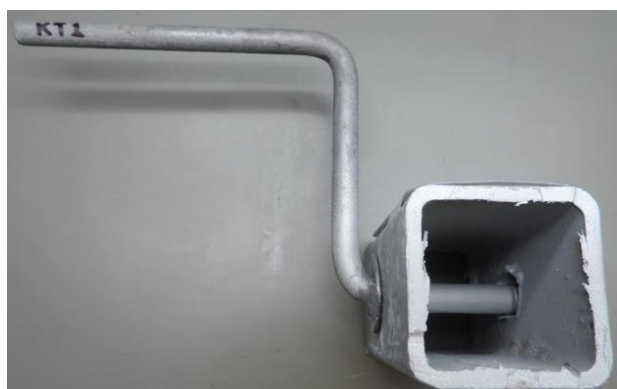
Figure 12. The appearance of the hook sets, before the salt spray test
