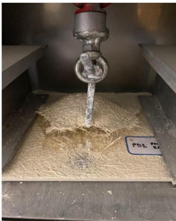
Figure 11. No rust was observed on embedded parts after severe corrosion
