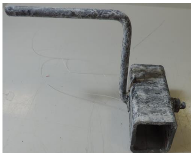
Figure 15. The appearance of the hook sets after the 96 th hour interim control
