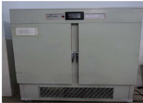
Figure 3. Atmospheric steam curing machine (steam chamber).
