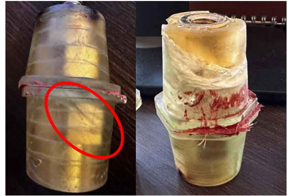
Figure 9 \pm 45^\circ fiber-reinforced specimen after test
