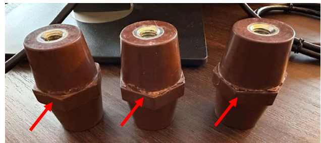
Figure 15 Silica filled purchased specimens after tensile test
