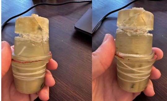
Figure 11 Fiber direction parallel to tensile load specimens after test
