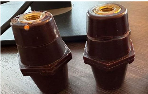
Figure 17 Silica filled inhouse specimens after tensile test
