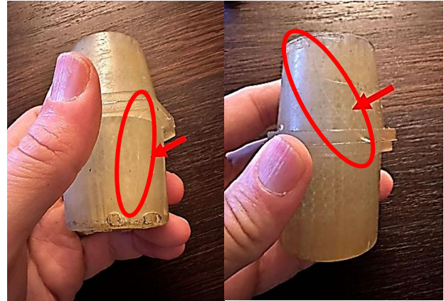
Figure 13 Fiber direction perpendicular to tensile load specimens after test
