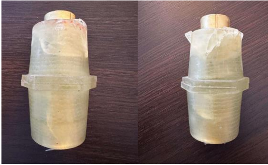
Figure 7 \pm 90^\circ fiber-reinforced specimen after test
