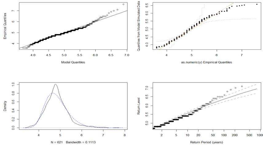
Figure 7. Diagnostic plots and return level analysis for earthquake magnitude data using the generalized extreme value distribution.
