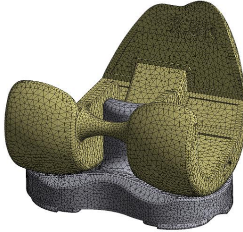
Figure 5. Finite element model of the implant used in the analysis (Ozer, 2022)
