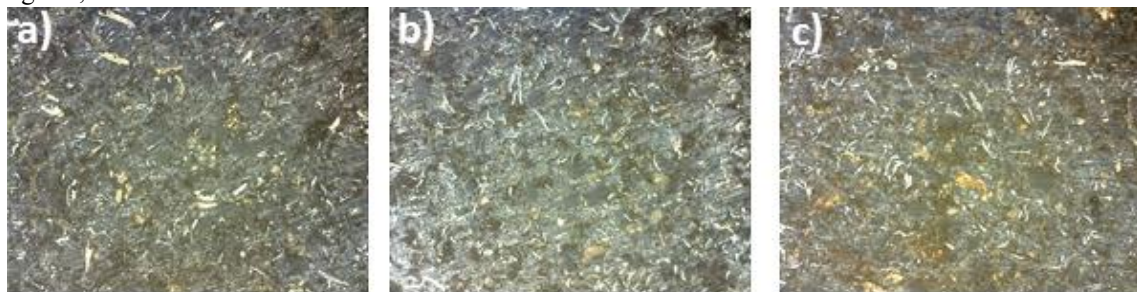
Figure 7. Microstructure of hazelnut dust brake pads: (a) B-W, (b) B-C-W, (c) B-CYC-W
