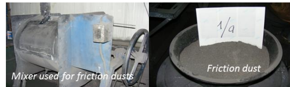
Figure 2. Mixer used for friction dust and friction dust
