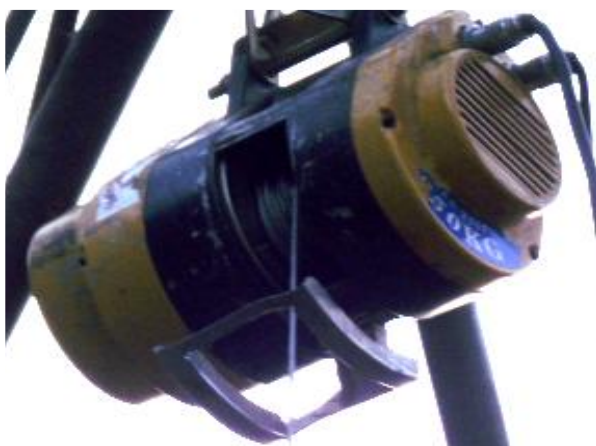
Figure 4. “Biglift” electric powered winch and remote control device
