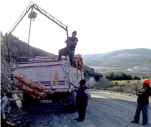
Figure 3. Electric powered winch loading
