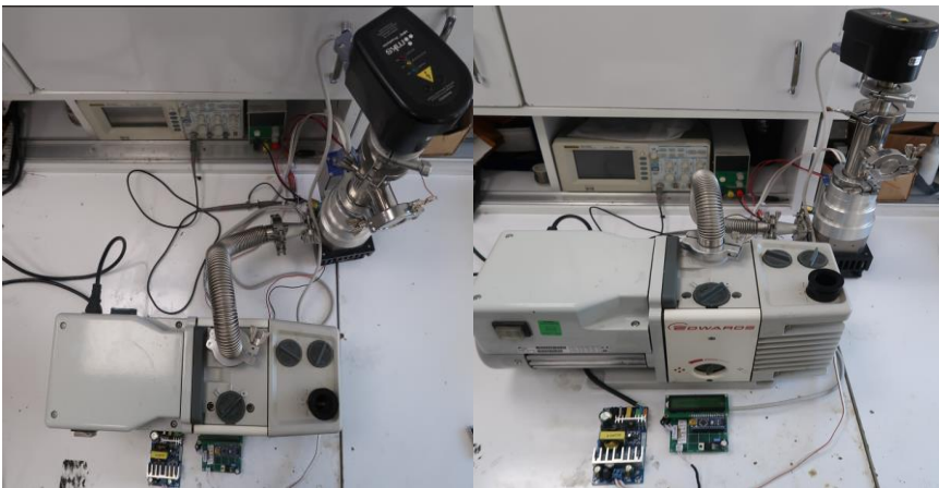
Figure 9. Experimental Setup for Vacuum Measurement
