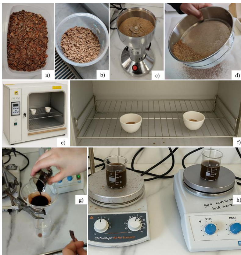
Figure 1. Preparation of shell powders: (a) hazelnut, (b) walnut, (c) grinding, (d) sieving, (e – f) heat treatment, (g – h) surface modification.
