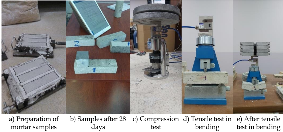
Figure 5. Lime mortar material tests
