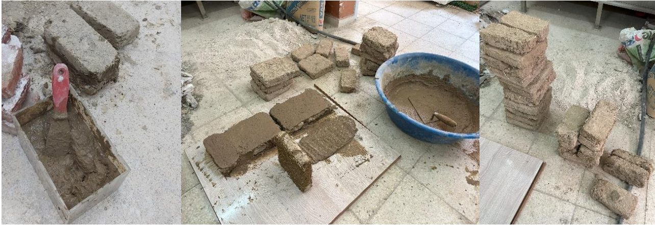
a) Adobe mortar production b) Preparation of multilayer adobe specimens c) Cap making
