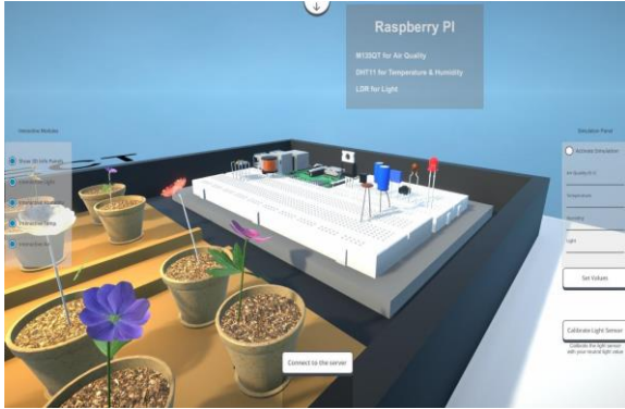
Figure 3. Interactive digital twin scene developed in Unity 3D for real-time greenhouse monitoring and control
