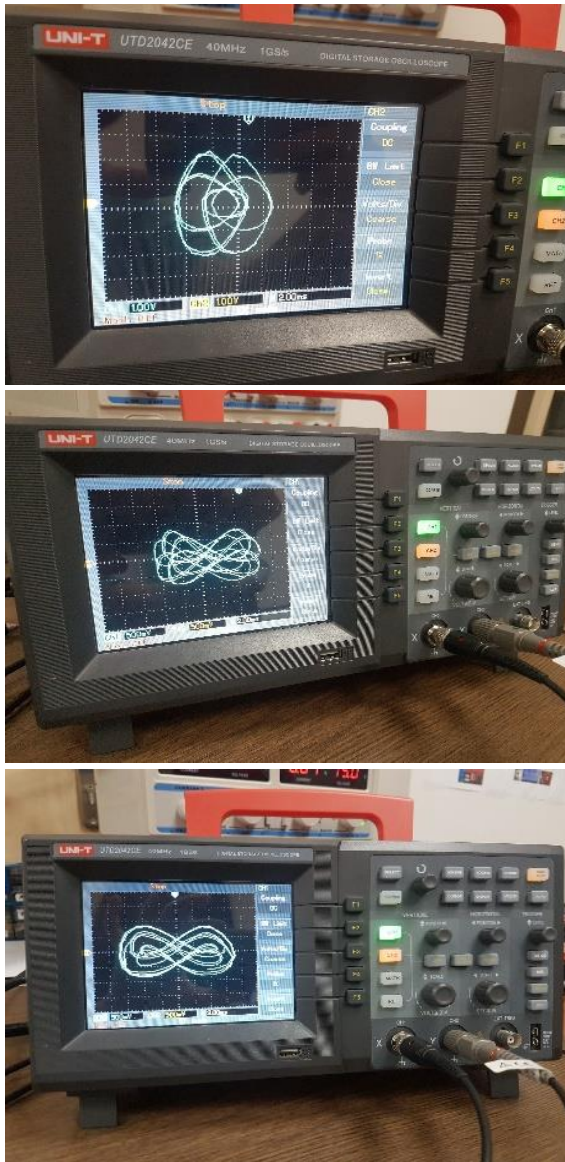
Figure 10. Oscilloscope images of the system's phase portraits.
