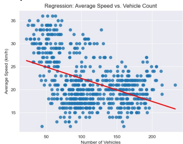
Fig. 9. OLS regression: Average speed vs Vehicle Count
