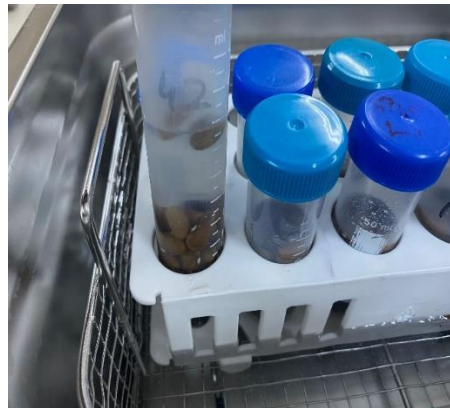
Figure 4. Ultrasonic sound wave application to bean seeds
