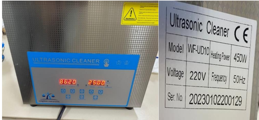
Figure 3. Ultrasonic sound wave application device
