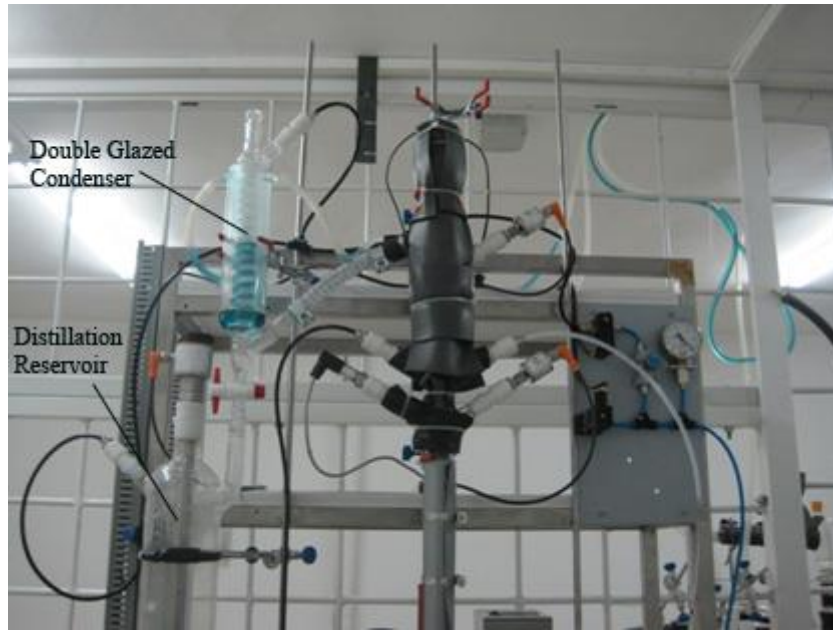
Figure 3. Double glazed condenser and distillation reservoir.
