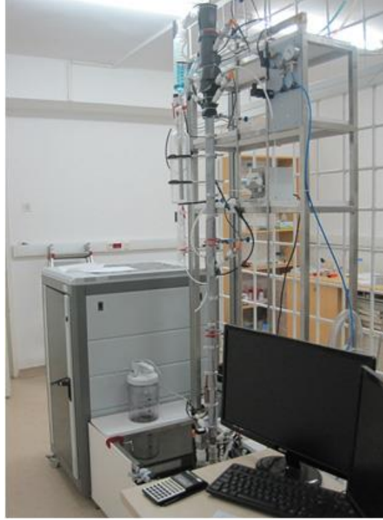
Figure 2. Filled Tray Type Column System.
