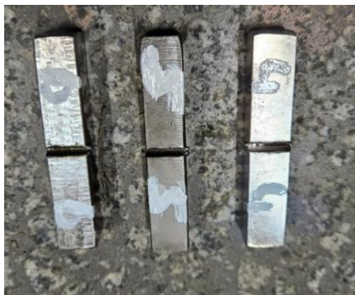
Figure 7. The samples after Charpy test at -70 degrees Celsius
