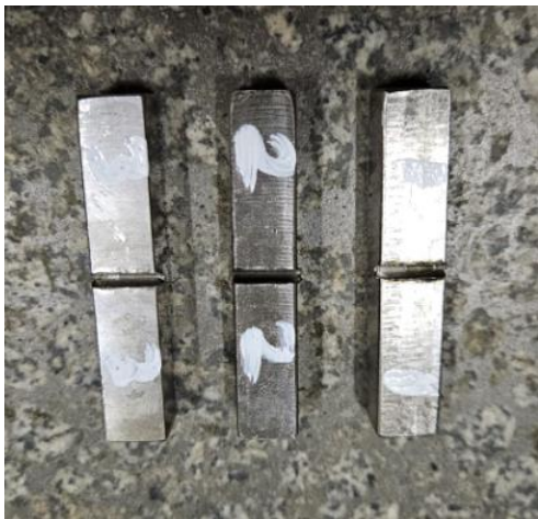
Figure 6. The samples after Charpy test at room temperature
