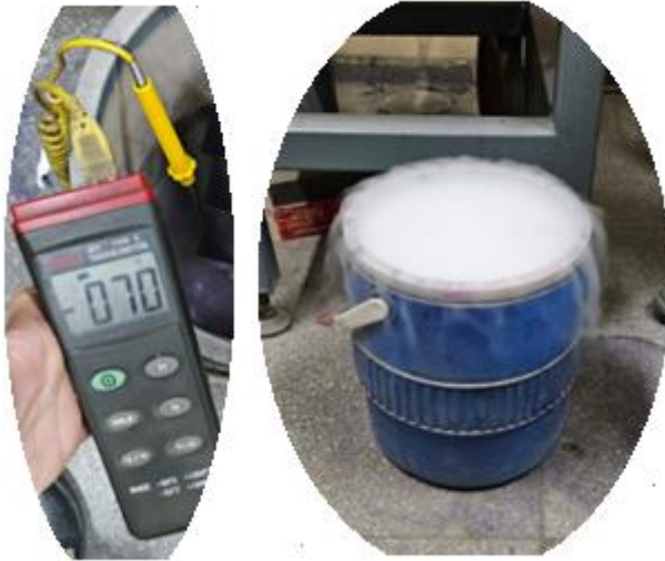
Figure 5. Preparation of the Charpy test samples in -70 °C
