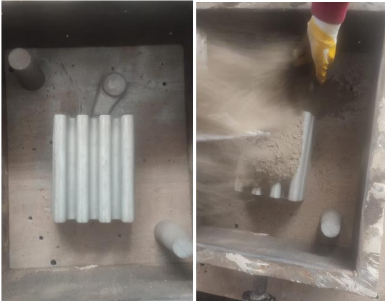
Figure 1. Placing the model in the sand
