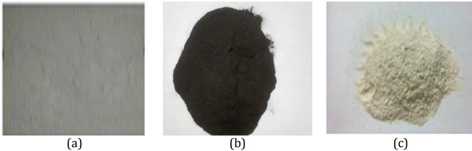
**Fig. 1** Photographs of the raw materials for (a) 150 µm silicon carbide particles, (b) 150 µm millscale particles, and (c) received 53 µm magnesia particles.
