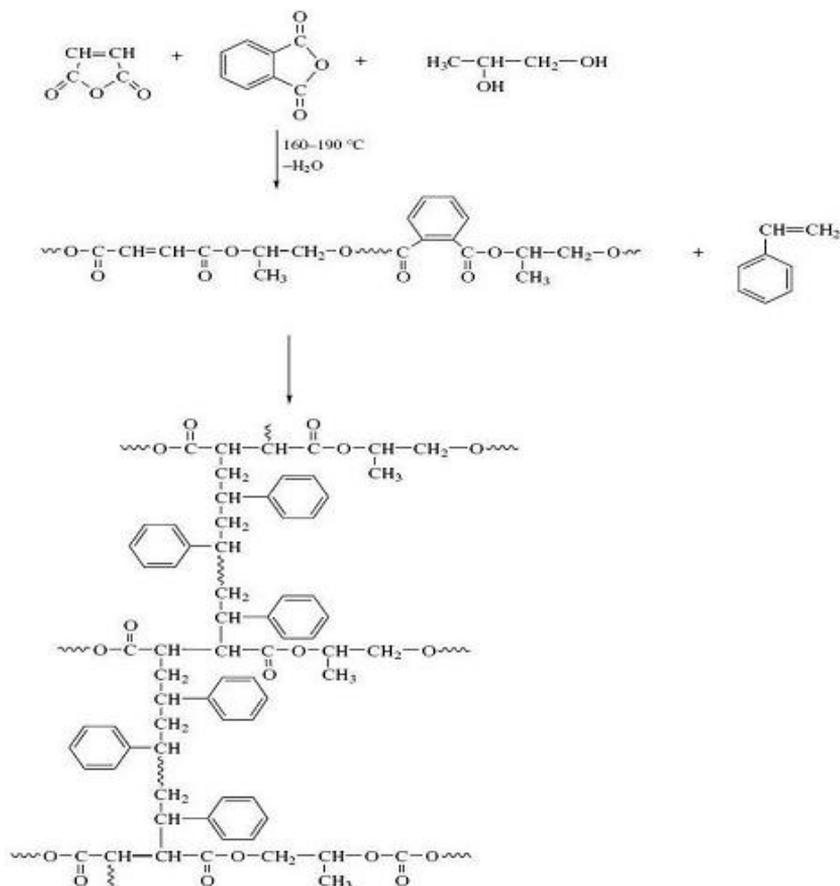
**Fig. 2** Chemical structure of a typical unsaturated polyester resin linkage [7].
