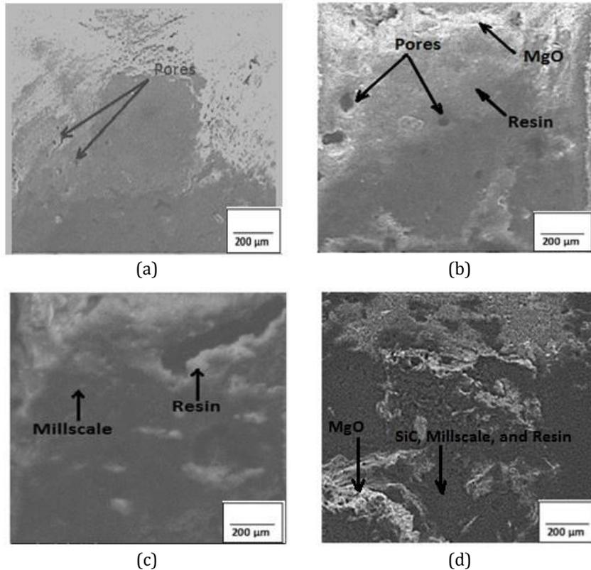
**Fig. 3** Microstructure of the samples for (a) unreinforced unsaturated resin matrix, (b) 15 wt. % MgO particles reinforced, (c) 15 wt. % Mill-scale particles reinforced, and (d) 15 wt. % hybrid composites.
