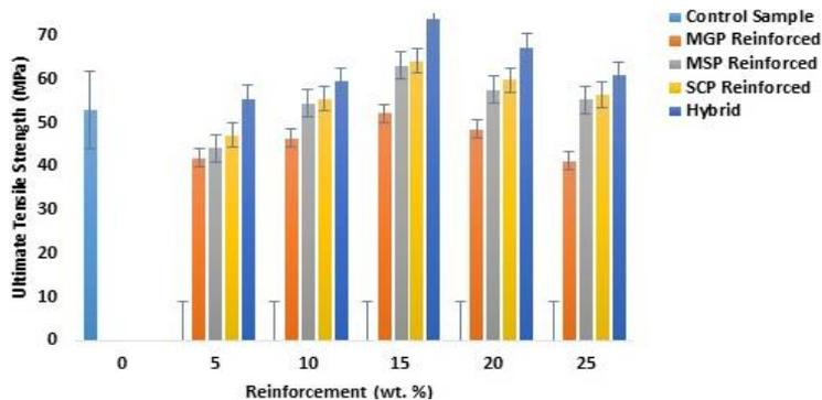
**Fig. 4** Graph of ultimate tensile strength against wt. % reinforcement of the composites.
