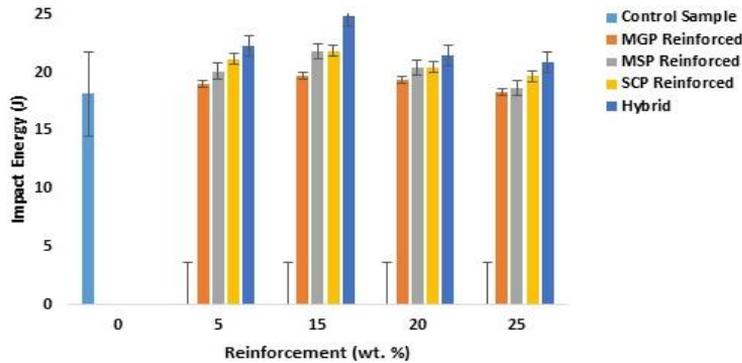
Fig. 7 Graph of impact energy against wt. % reinforcement of the composites.
