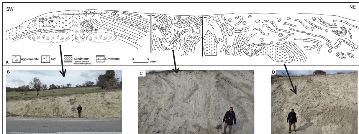
Figure 7- Chaotic structures, a) geological cross section showing chaotic structures, b) agglomerate blocks and slump structures, c) slump structures affecting the bedded limestones and tuff clastics, d) tuff block and slump structures.
