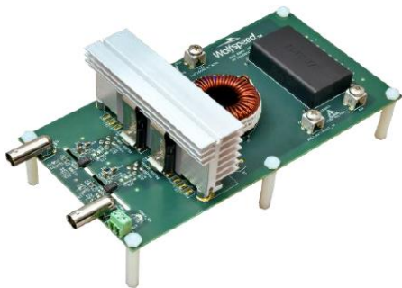
Figure 3. SiC mosfet based DC-DC converter
