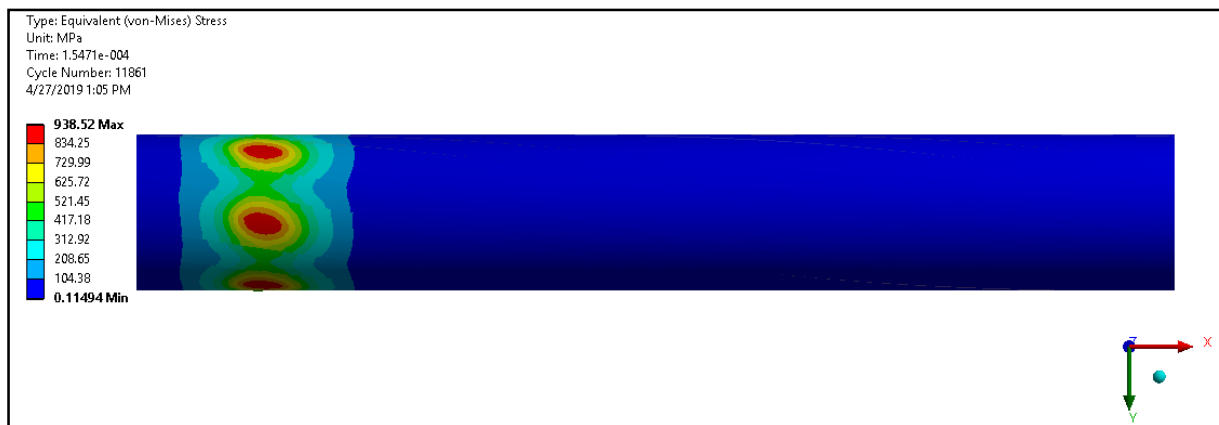
Figure 17. Maximum equivalent stress formed on the outer surface of the barrel ( t=154 \mu\text{s} )
