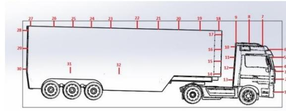
Figure 6. The location of the pressure probe on model car [2]
