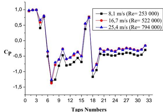
Figure 7. The pressure coefficient ( $C_p$ ) distribution on the truck trailer combination [2]
