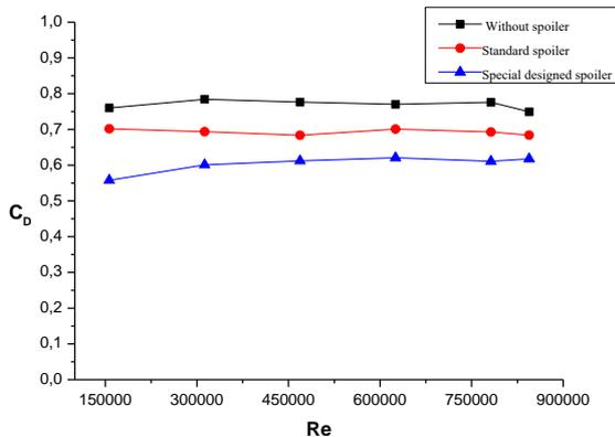
Figure 14. The drag coefficient graph of without spoiler-standard spoiler-new designed spoiler
