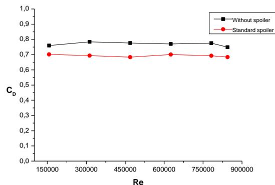
Fig.11. The drag coefficient graph of standard spoiler model (model 2)
