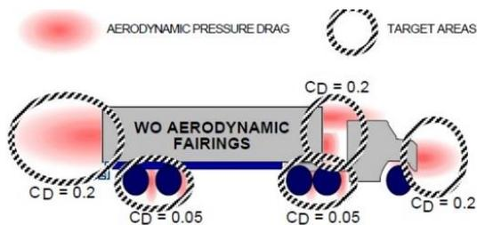
Figure 1. The high pressure resistance regions on heavy vehicles [1]
