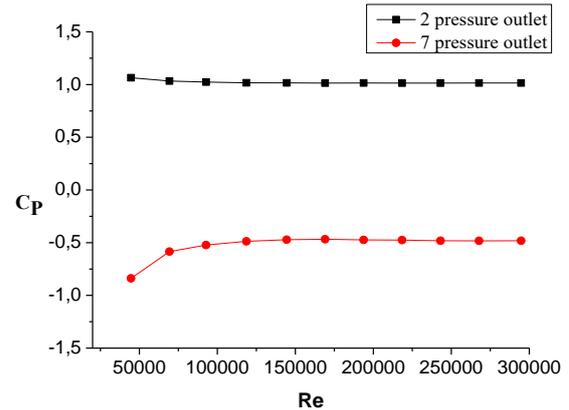
Figure 5. Reynolds independent in tests
