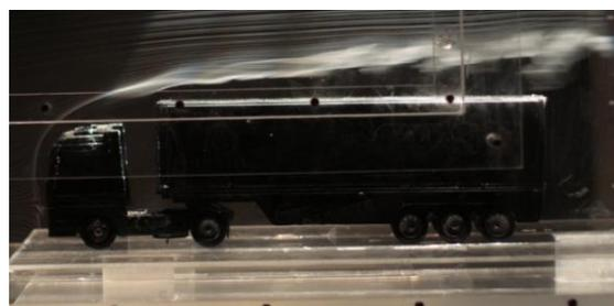
Figure 12. Flow visualization of model 2 [2]
