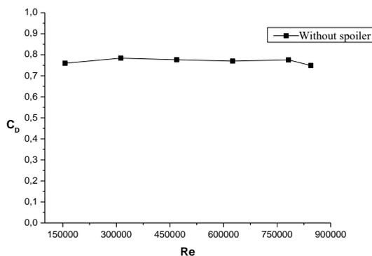
Figure 9. The drag coefficient graph of without spoiler model vehicle (model 1)
