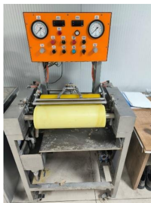
Figure 2. Laboratory-type Surface Application Sizing Press Unit.
