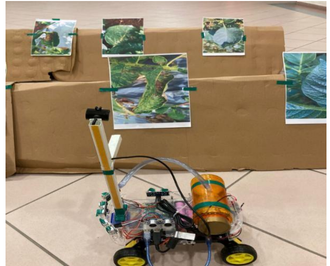
Fig.23. Detecting and Spraying Simulations by the UGV
