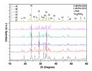
**Figure 2.** X-ray powder diffraction patterns of (BiPb)<sub>2</sub>W<sub>x</sub>Sr<sub>2</sub>Ca<sub>3</sub>Cu<sub>4-y</sub>Mo<sub>y</sub>O<sub>12+&</sub> superconducting samples. (L) Bi-2212 phase,(H) Bi-2223 and (\*) Ca<sub>2</sub>PbO<sub>4</sub> secondary phase.
