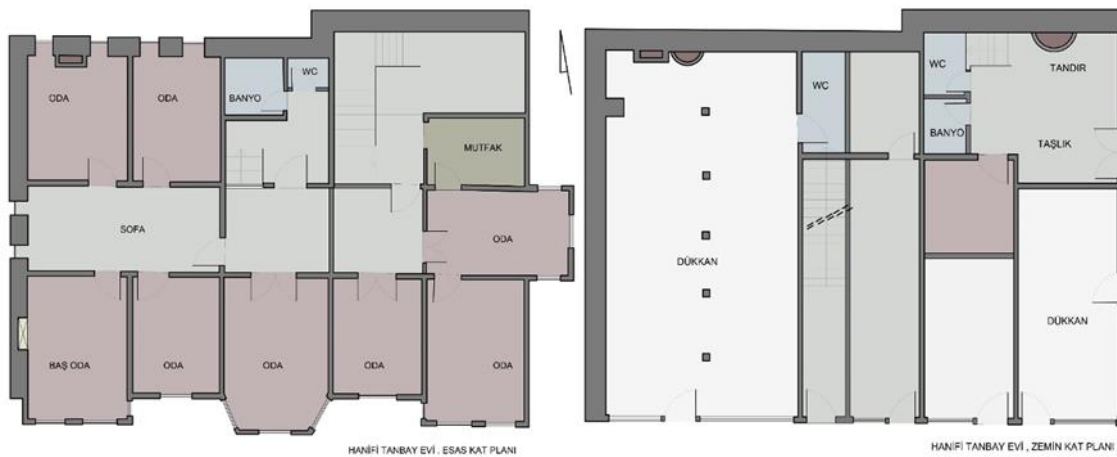
Figure 9. Plan of the Hanifi Tanbey House (Adapted by the authors based on the drawings of Temiz, 1990)
