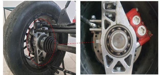
Figure 2. Close-up images of the rear upright assembly, showing the integration of the wheel hub, bearing housing, brake caliper, and suspension linkage interfaces.
