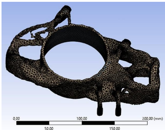
Figure 8. Optimized geometry of the upright component after topology optimization.
