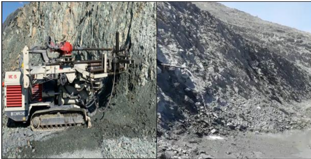
Şekil 16. Sahada kurulan yatay delgi makinesi ve yatay kuyudan gelen su örneği (Horizontal drilling machine set up in the field and water sample taken from horizontal well)
