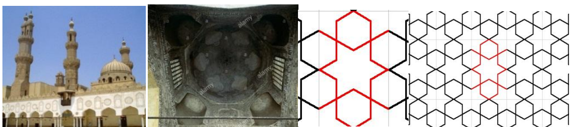
Figure 7: Al-Azhar Mosque and the detail of the dome showing a six point geometrical pattern (Tentoila, 2006) The pattern tessellation drawn by authors
