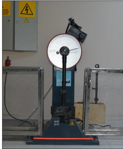
Figure 7. Charpy impact tester.
