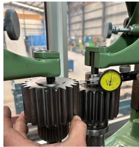
Figure 16. Measurement of the Backlash Distance
