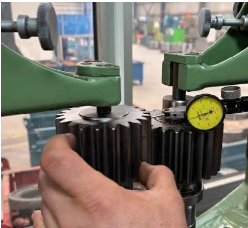
Figure 15. Zeroing of the Backlash Distance
