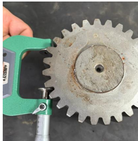
Figure 14. Sun gear 4 teet measurement
