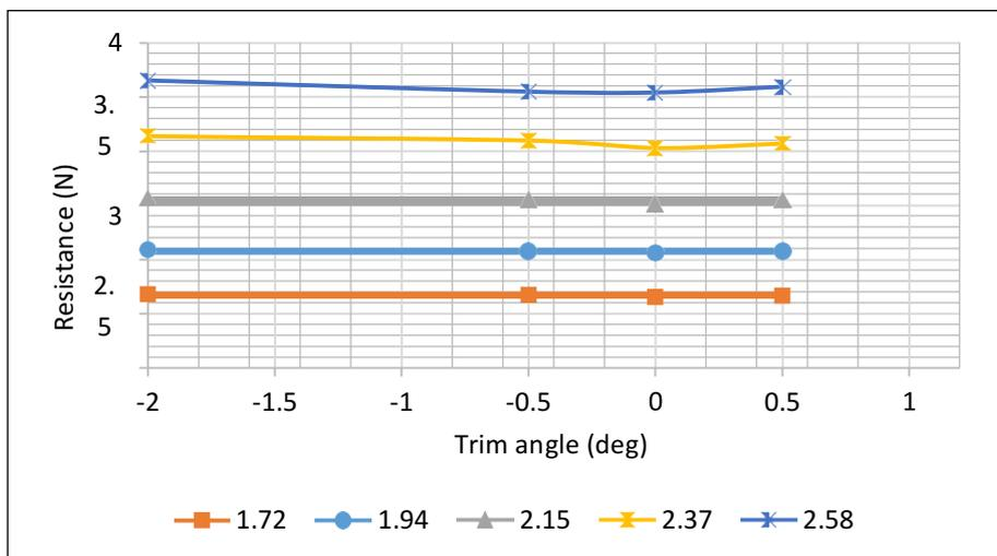
**Fig. 6.** Results from the CFD: Resistance of the rowing eight’s shell at various speed and trim.
