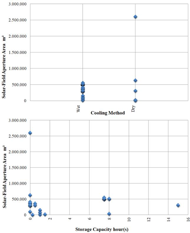
**Fig. 3.** Inputs and outputs (top to bottom): DNI, engineering design year, net installed power, cooling method, storage capacity versus land area and then solar field aperture area (see ESM) (generated by Microsoft Office Excel 2007 or Apache OpenOffice 4.1.5 & Paint.NET), Data: [56].
