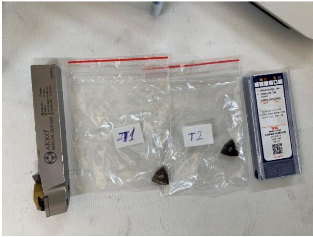
Figure 6. A photograph of the cutting insert and cutting tool holder used in the machining experiments.
