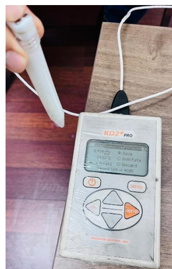
Figure 4. A view of measurement process made with KD-2 Pro thermal conductivity measurement device.
