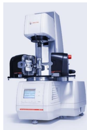
Figure 3. A photograph of Anton Paar brand MCR 702-e compact rheometer (Anton Paar Incorporation, 2023).
