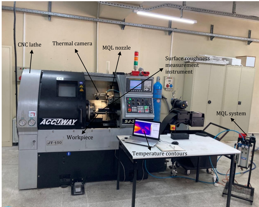
Figure 5. A photograph of the experimental setup for the machining.
