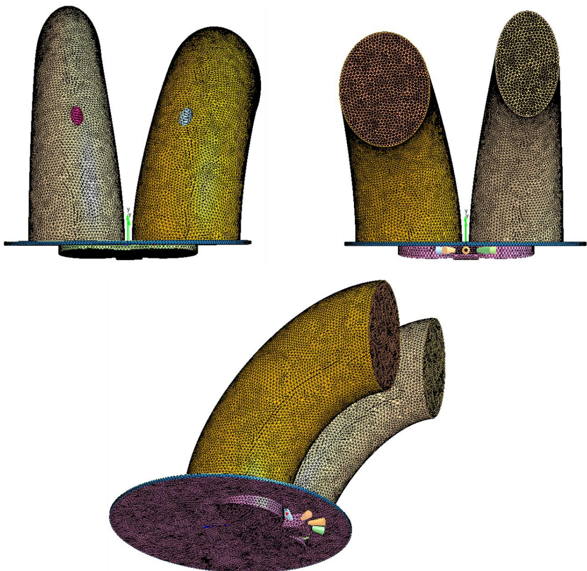
Figure 4. Mesh structure for 3D ICC CFD model of in-cylinder
