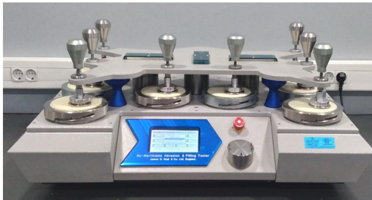
Figure 1. Martindale Abrasion and Pilling Test Device
