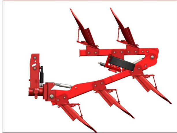
Figure 4. Hydraulic folded reversible moldboard plow (Original).
