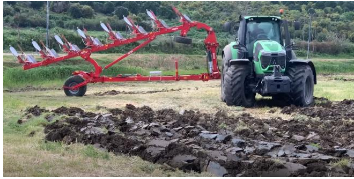
Figure 3. Semi mounted- trailed type reversible plow end of field turn.
