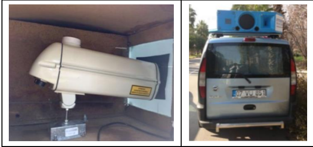
Figure 8. Average speed cameras setup placed on the vehicle (average speed camera&camouflage within luggage) [43],[65].
