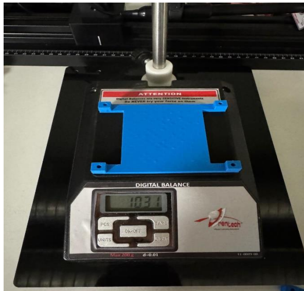
Figure 9. The 3D-printed version of the robot chassis modeled prior to topology optimization
