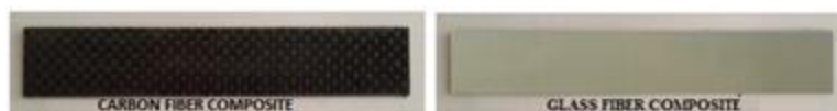
Figure 5. Carbon fiber composite material and glass fiber composite material prepared for the determination of mechanical properties
