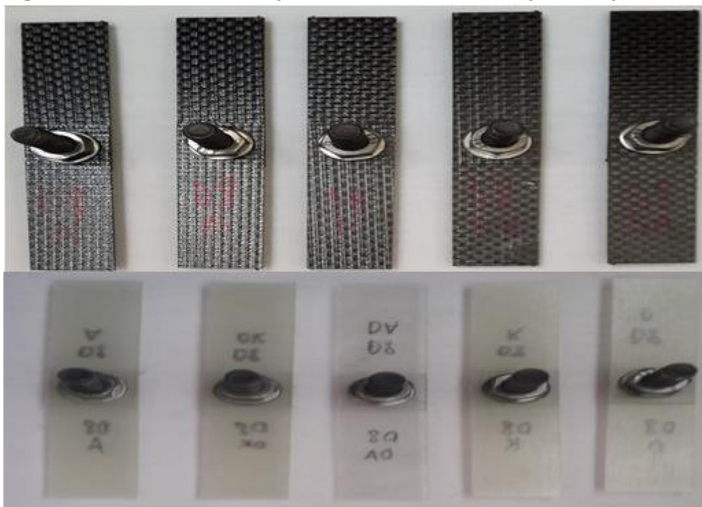
Figure 3. Carbon fiber composite materials and glass fiber composite materials joined together using bolts
