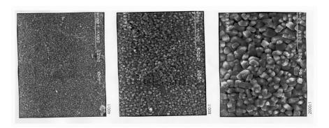
Zinc Phosphate Coating Crystal Structure (Scanning Electron Microscope)
